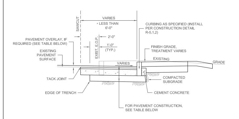
\* NOTE: FOR PROPOSED WIDENING OF 6 FEET OR GREATER IN WIDTH, SEE CONSTRUCTION DETAIL R-5.1.5
